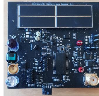
**Figure 1: Battery-free polymorphic light sensor.** We can sense ultraviolet, infrared, blue and visible light, and communicate them using a backscatter mechanism. We can operate solely on harvested energy, which is obtained using a small sub-credit card-sized solar cell and stored in a capacitor.
