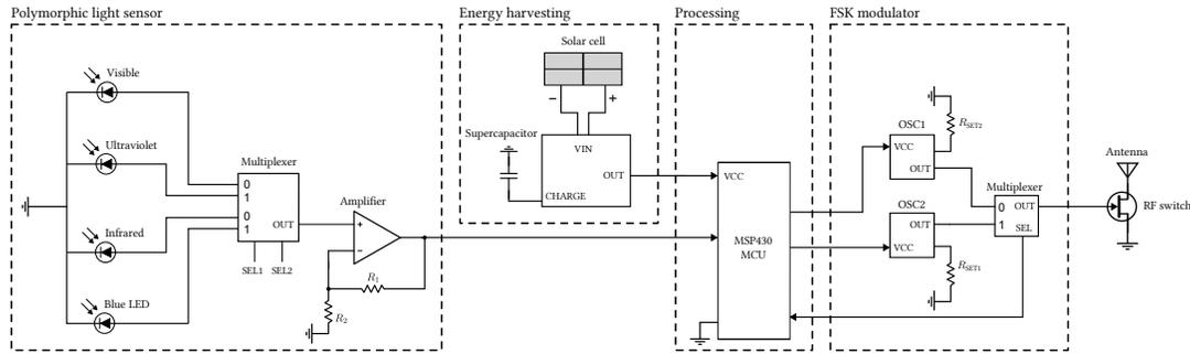
**Figure 2: Battery-free Polymorphic Light Sensor.** Combining photodiodes and LEDs with sensitivity to different parts of the light spectrum enables us to sense broad light spectrum. Operation in photo-voltaic mode enables operation on the harvested energy. Light sensor readings are communicated using ultra-low power backscatter communication built using LoRea.
